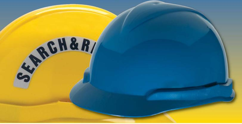
Vanguard<sup>™</sup> Caps are designed to provide limited impact and penetration protection in the event of a top or lateral blow to the head. These caps meet all applicable requirements for a Type I and II (top and lateral impact) helmet as outlined in ANSI/ISEA Z89.1-2009 (Class E) and CSA Z94.1-2005 (Class E).
